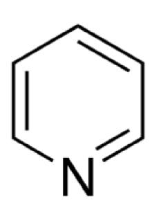
Product Name **Pyridine** Product Code C0861 CAS Number 110-86-1 Molecular formula  $C_5H_5N$ Linear formula  $C_5H_5N$ Molecular weight 79.10 Sensitivity heat, light Melting point -42C 115C Boiling point
